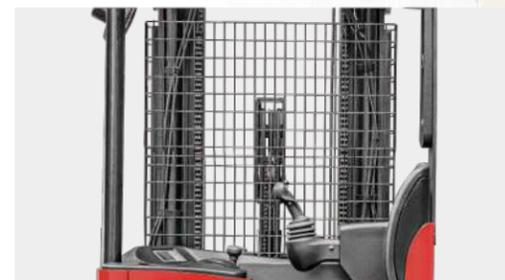
The Full Free Lift 3 Stage Mast provides great visibility for the operator, and improves operations safety.
