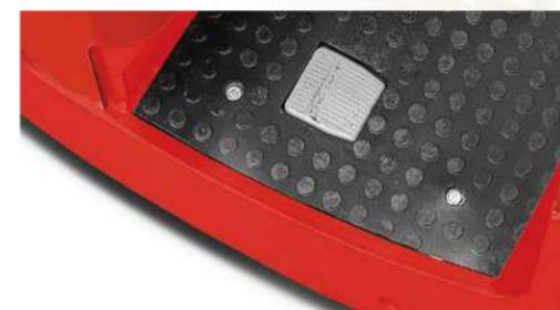
With the pedal sensing system, the truck can be driven only if the driver stands on the pedal. If the operator takes their foot off the pedal, active braking is initiated to prevent an accident.
