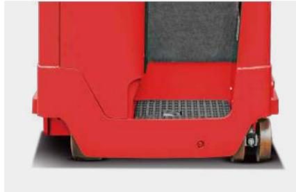
The operator is able to get on and off the truck more comfortably thanks to the low step-on height of the reach truck's operator compartment.
